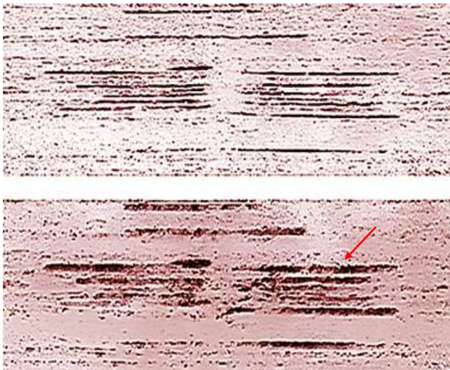
Fig.( 3). Gate width's effect on the accuracy of backscattered echoes' crack imaging. Gate widths are as follows
